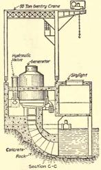
Fig. 306.—Section C-C. Through the generator platform.
